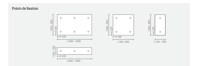
Quadrillage de fixatioan
